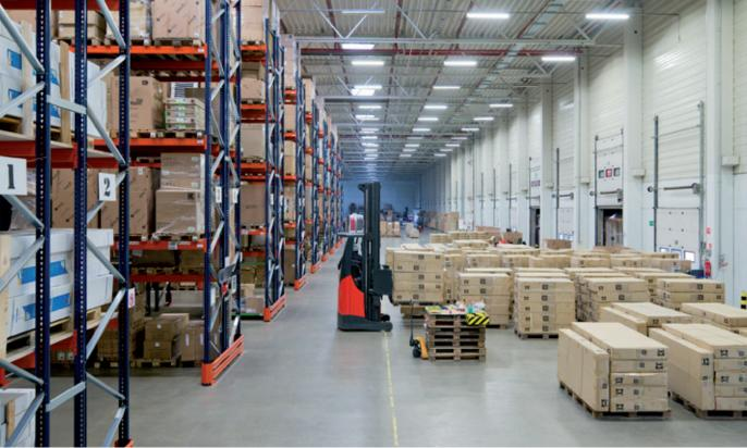
HSF e-commerce has equipped its logistics centre in Sady (Poland) with 122 m long Mecalux pallet racks that provide a storage capacity for 11,592 pallets. More than 10,000 SKUs of different volumes and dimensions are managed in this warehouse. The direct access to the racks quickens storage tasks and prep of 2,000 orders a day.
